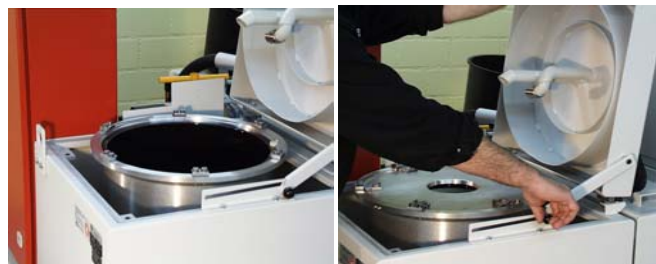
Re-install rotor cover and close housing cover, secure the lock catches and switch on centrifuge.
