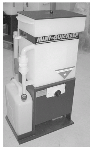
MINI-QUICKSEP MK II 120 with 10 l oil tank.
