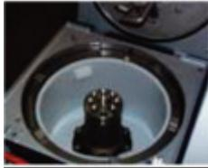
Remove the insert filled with slurry.
