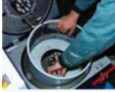
Insert a cleaned slurry insert.
