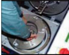
Refit the rotor and the housing cover (lock the quick-release fasteners) and restart the centrifuge.
