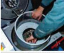
Insert a cleaned slurry insert.
