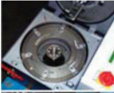
Switch off the centrifuge, open the housing cover and remove the rotor cover (release the quick-release fasteners).
