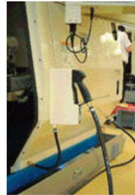
Gun in holster mounted on outside of machine
