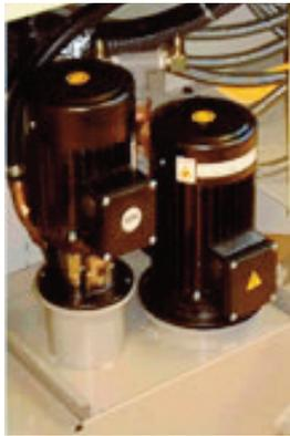
Delivery pump mounted in coolant tank
