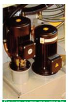
Delivery pump mounted in coolant tank
