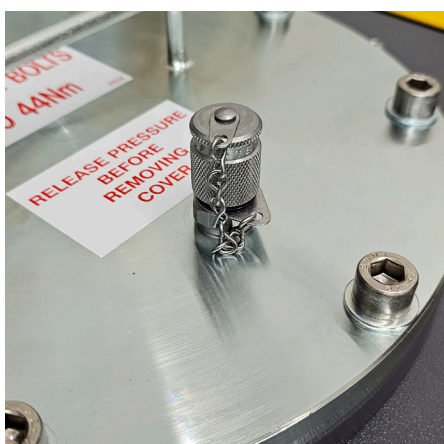
Step 6: Ensure the pump has stopped before removing the purge hose. Replace the protective filter port cap.
