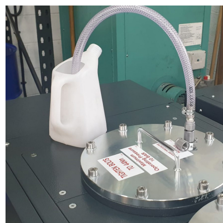
Step 5: When the jug has started filling, press the red standby button (below the green button). The filter has now been purged successfully.
